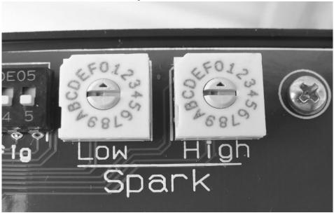
Be careful with these settings! Make sure you are monitoring for knock. These settings add or subtract from you chip's base timing if you have a compatible chip. "Low" is Opsi boost and lower, "High" is 10psi boost and higher (full throttle).
